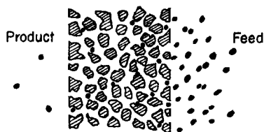
FIG. 2. Cross section of ultrafiltration membrane.
